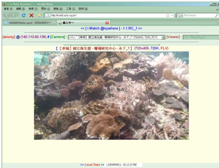
Fig. 3 A Web interface for stream viewing, users can select multiple real-time streams from top panel
